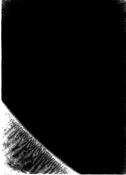
FIG. 13. Curved line defects. The photograph shows a stripe pattern permeated by an array of line defects emerging from the edge of the film (part of the filmholder is visible in the lower left portion of the image). Note that the cusps associated with successive defects adopt identical orientation (pointing upward). What are initially transverse line defects convert into longitudinal defects via “faceted” curved segments. A portion of a loop is visible in the lower right of the image. Details of the intensity modulations and cusp orientations are discussed in the text. The horizontal dimension of the field of view is approximately 180 \mu\text{m} .
